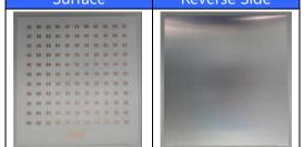
**Board: Aluminum (Copper foil on one** surface) Board Thickness: 1.0mm Copper Foil Thickness: 35µm Insulating Layer Thickness: 120µm
