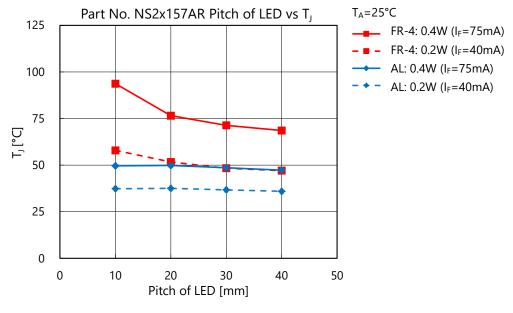
Figure 5. Junction Temperature at Each Pitch (Part No. NS2x157AR)
